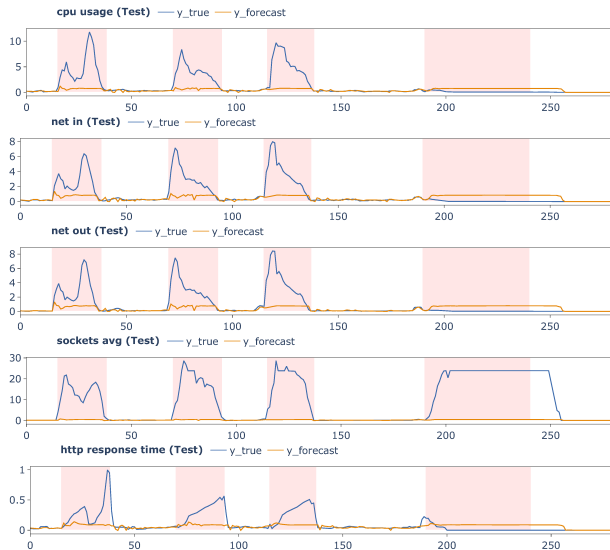
Fig. 6: Forecasting on testing data of the video streamer CNF of vCDN slice 1. The three first highlighted red regions correspond to Hulk attacks, while the last region represents the Slowloris attack.
