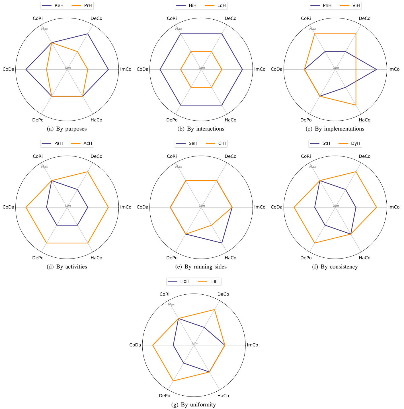
Fig. 2. Comparing the honeypot types in each class regarding Implementation Cost (ImCo), Design Complexity (DeCo), Compromising Risk (CoRi), Collected Data (CoDa), Deception Power (DePo), and Handled Connections (HaCo).
