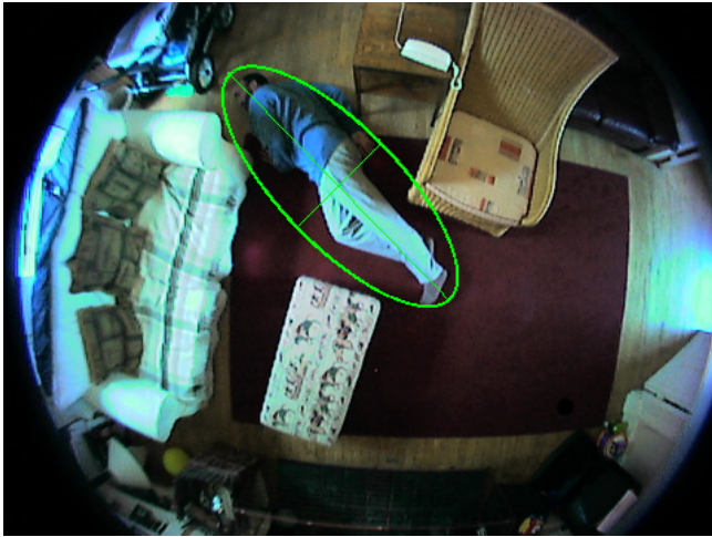
Fig. 10. An example of fall where HM detects the occupant being inactive in an unusual location.
