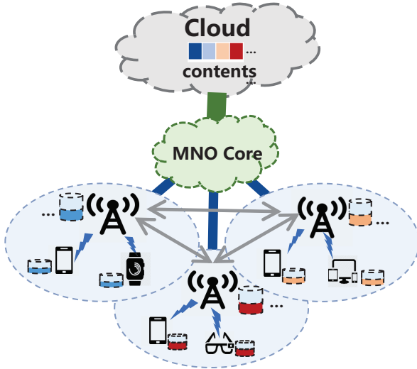
Fig. 1. Cooperative edge caching-supported IoT architecture.
